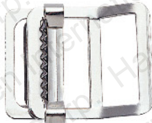
635S Sheet Steel Buckle Thickness: .039", .039", .047", .047", .063" Size: 1/2", 5/8", 3/4", 1", 1 1/2"
