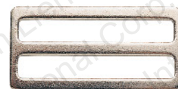
5048 Sheet Steel Size Thickness Slot 1 1/4" .09" .311" 1 1/2" .09" .268" 2" .09" .311"
